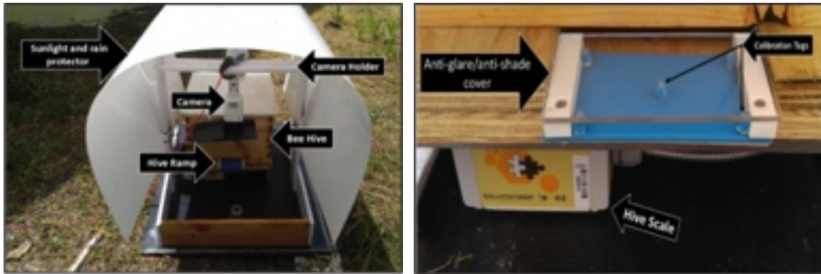
Large-scale recording of bee activities 24/7 using cameras and sensors
